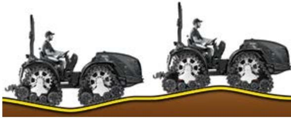
Thanks to the 45° offset of the front and rear axle final drives, the Mach 4 combines a long wheelbase with a reduced engine overhang: features which grant perfect stability in all operations, ensuring maximum safety and comfort at all times.
