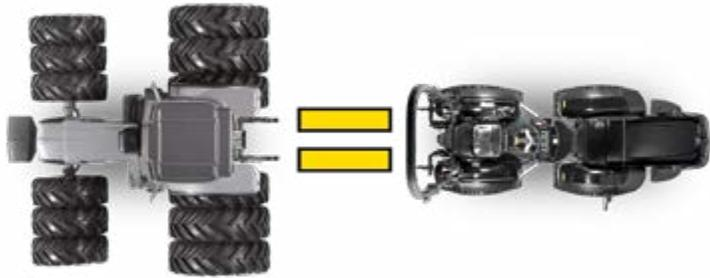
The four alternate-grip rubber tracks (w: 13,78 in), similar to "ground profile" tyres, assure constant adherence during all manoeuvres, even on slippery ground.
