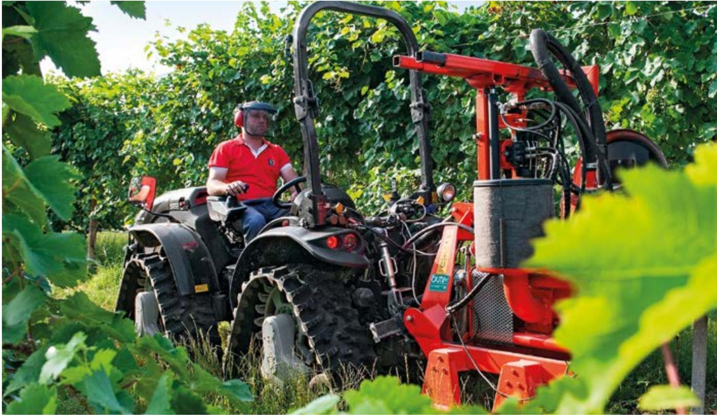
The lighting system, incorporated in the mudguards, features parabolic reflector units for a longer view of the track ahead, the implement and the surrounding area. Servicing is quick and easy thanks to the fully-opening bonnet and easily removable engine compartment side panels and battery cover.
