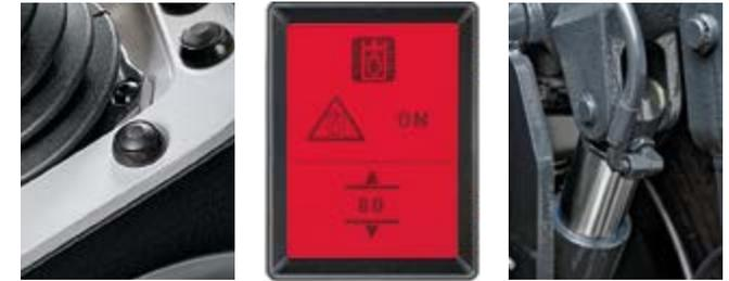
The Uniflex\* suspension with electronic control transfers part of the weight of the implement on the wheels. The reduced ground pressure has many benefits:
